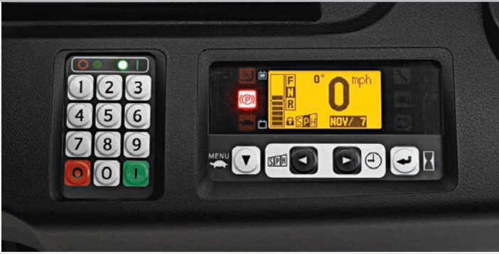
LCD Multifunction Display (STD) & Pin Code Entry System (OPT)
