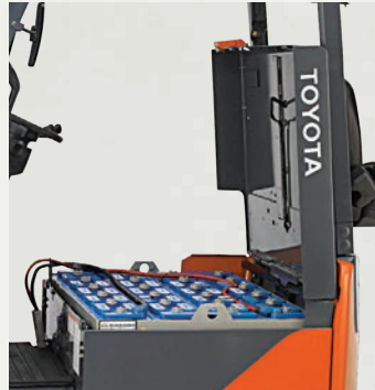
Heavy-Gauge, Formed-Steel Battery Compartment Hood
