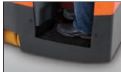
LOW 200MM STEP HEIGHT (200 mm 4150; 240 mm 4250)
